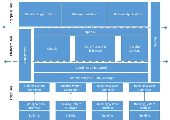
Fig. 2. TOPAs Open BMS Reference Architecture: Functional Model
